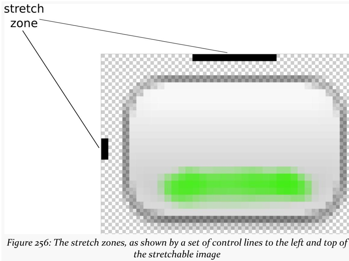
*Figure 256: The stretch zones, as shown by a set of control lines to the left and top of the stretchable image*
