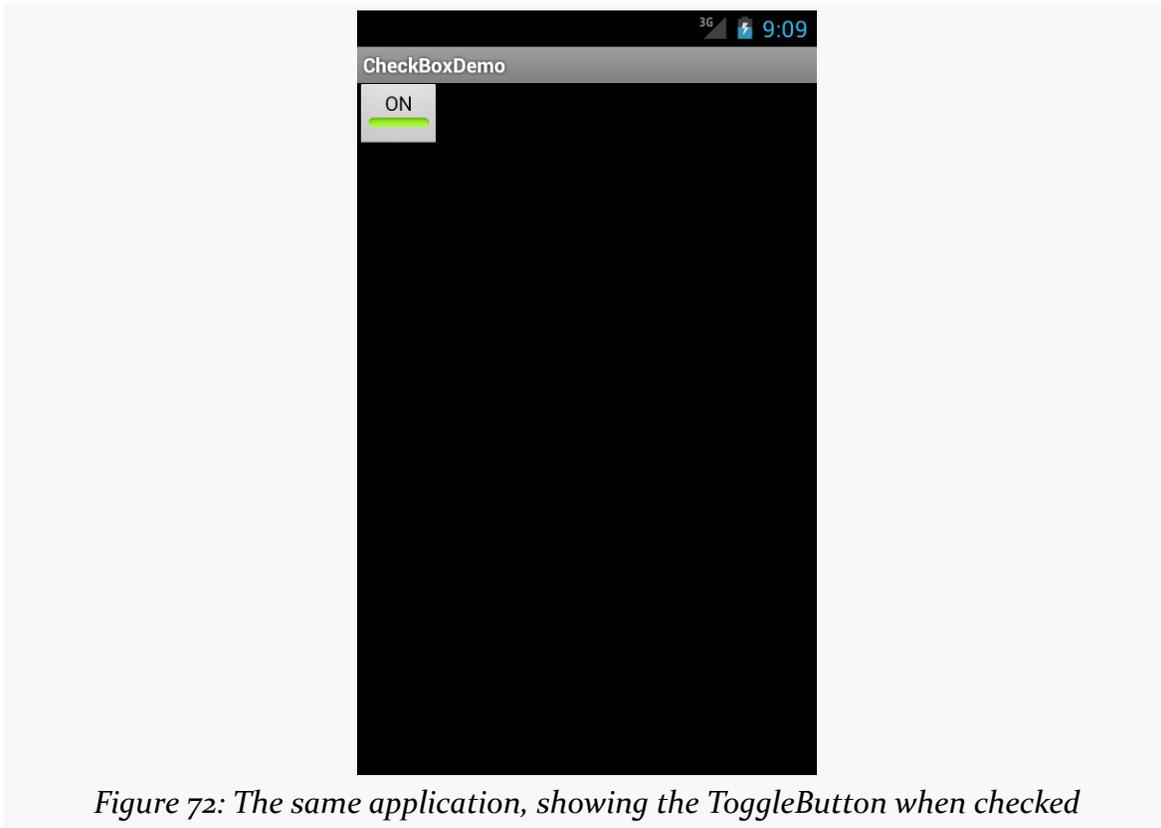
Figure 72: The same application, showing the ToggleButton when checked
