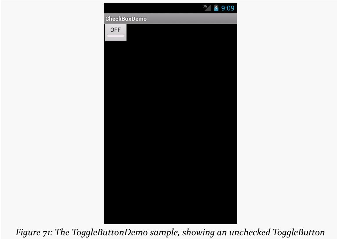
*Figure 71: The `ToggleButtonDemo` sample, showing an unchecked `ToggleButton`*
