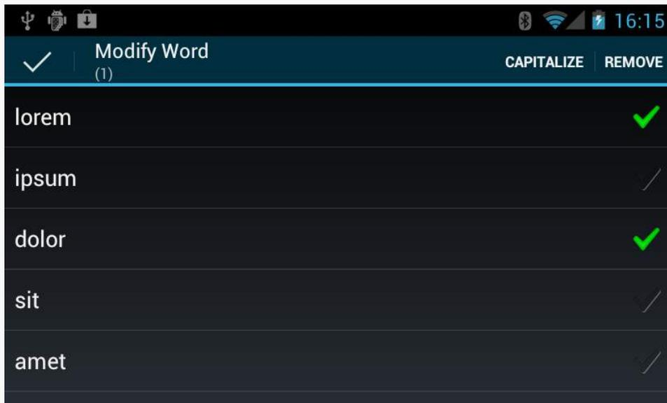
Figure 235: The `ActionModeMC` sample on a phone, using a split action bar, in landscape orientation
