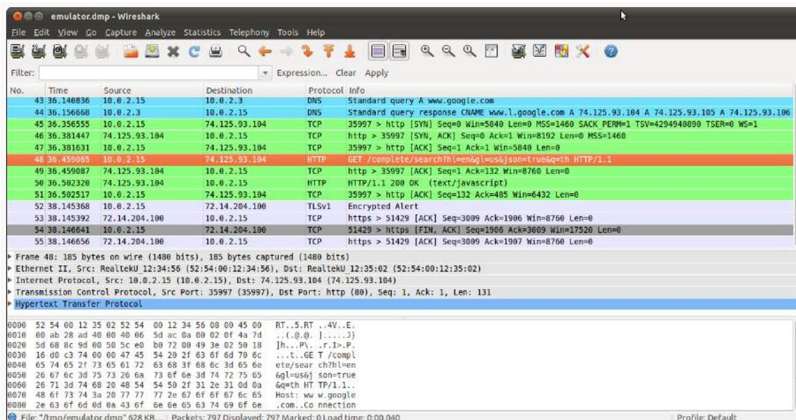
Figure 406: Wireshark examining captured emulator packets
