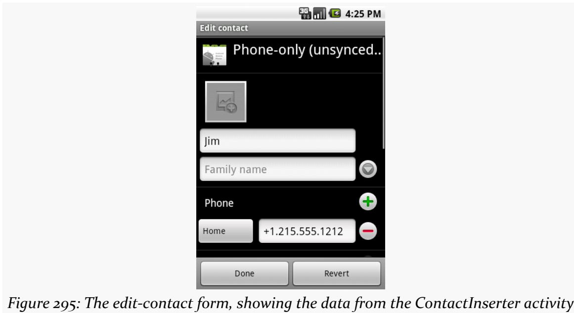
*Figure 295: The edit-contact form, showing the data from the ContactInserter activity*
