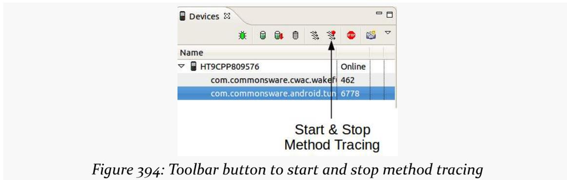
*Figure 394: Toolbar button to start and stop method tracing*
