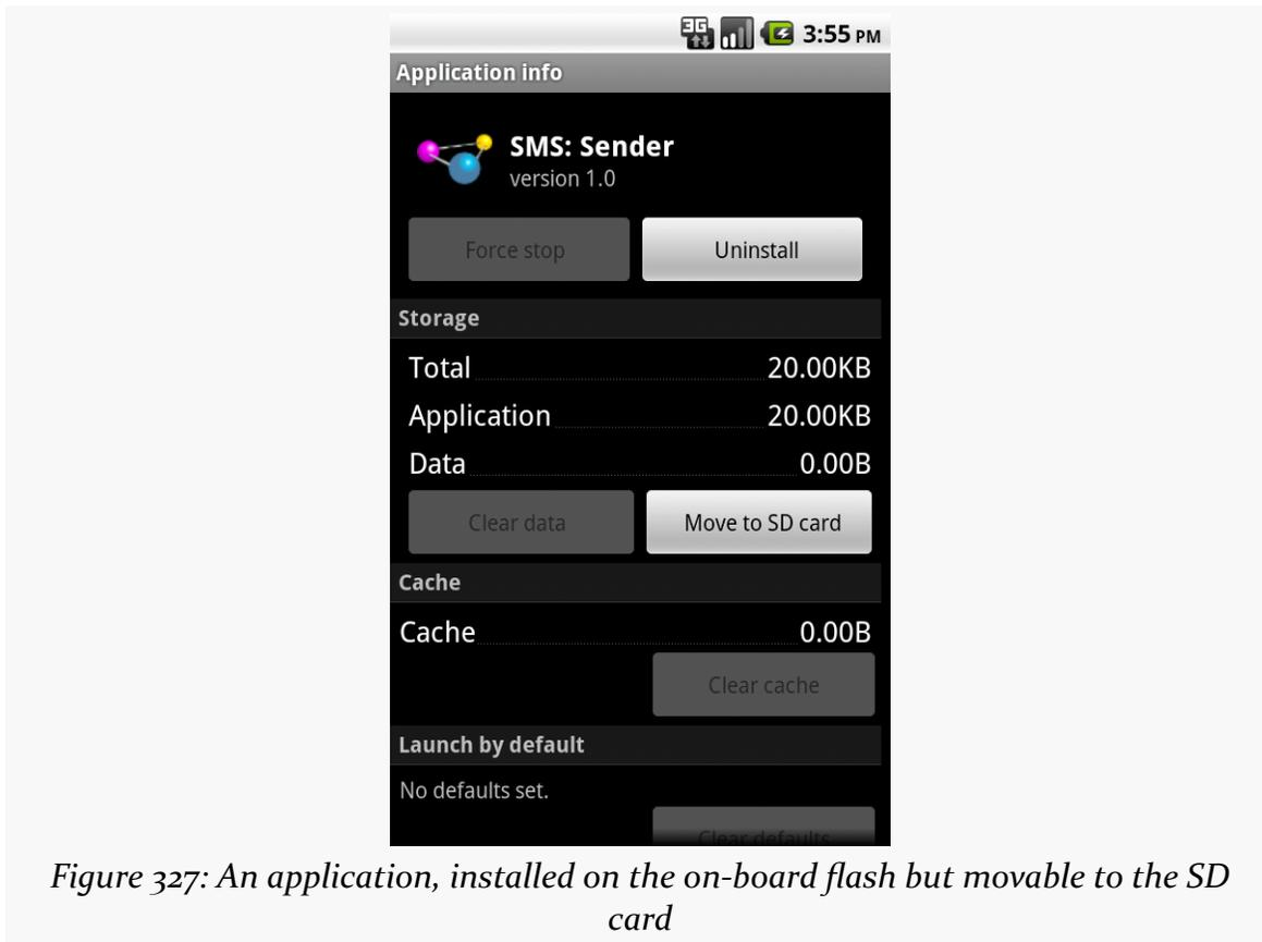
*Figure 327: An application, installed on the on-board flash but movable to the SD card*
